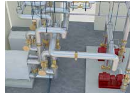
Before CR Equipment missing in mechanical plant room (Air separator, Expansion Tank Break Tank, Carbon Filter)
